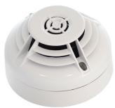
The sensing elements of the Opal NFX-SMT2 are panel controllable so the sensitivity thresholds of each element can be changed by the panel offering the ability to customise the device for the changing use of the area it is protecting. The detector has two integral tri-colour LEDs that provide 360° local visual indication of the device status. The LEDs are programmable with static or blinking red, amber and green status indications available.
